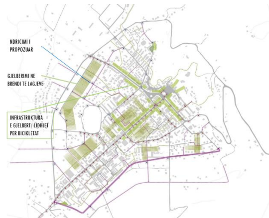
Figura 12: Proposed green infrastructure and lightning system
